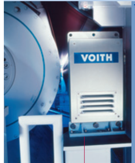
Fig. 2: Felt condition measurement.
