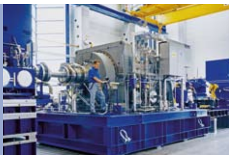
The largest Vorecon (33 MW) so far on the test bench in Crailsheim.
