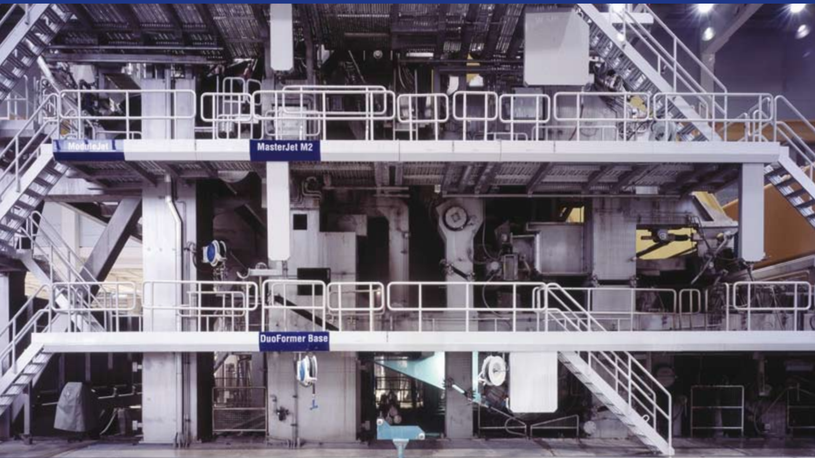
One of 40 gap formers for board and packaging papers running worldwide - DuoFormer Base at Jass Schwarza.
