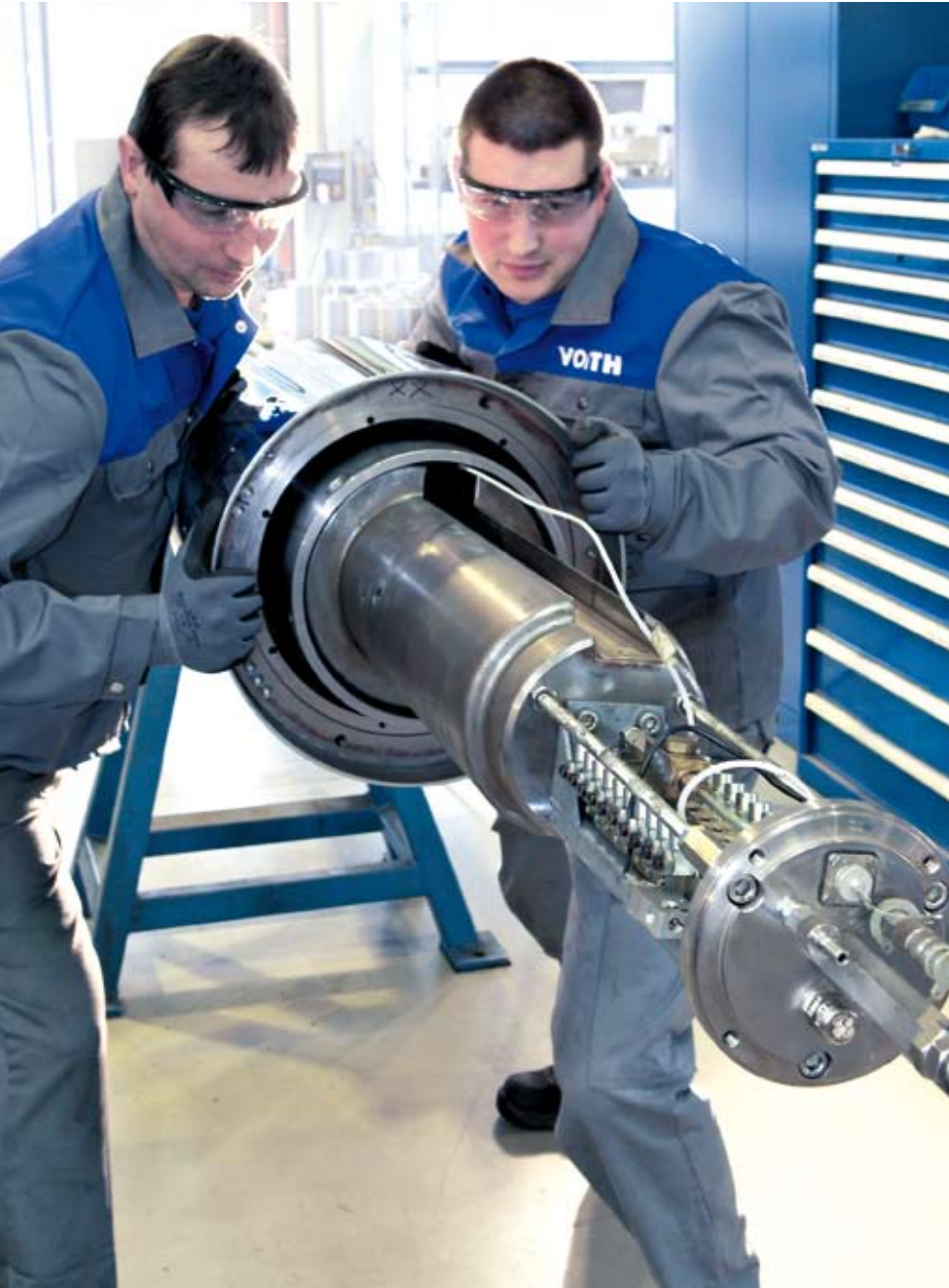
Disassembling of a spreader roll.
