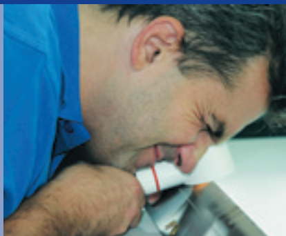
Checking blade wear traces on site to determine the optimal doctor setting
