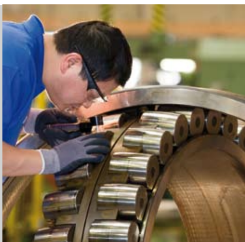
RollCare: Bearing inspection.
