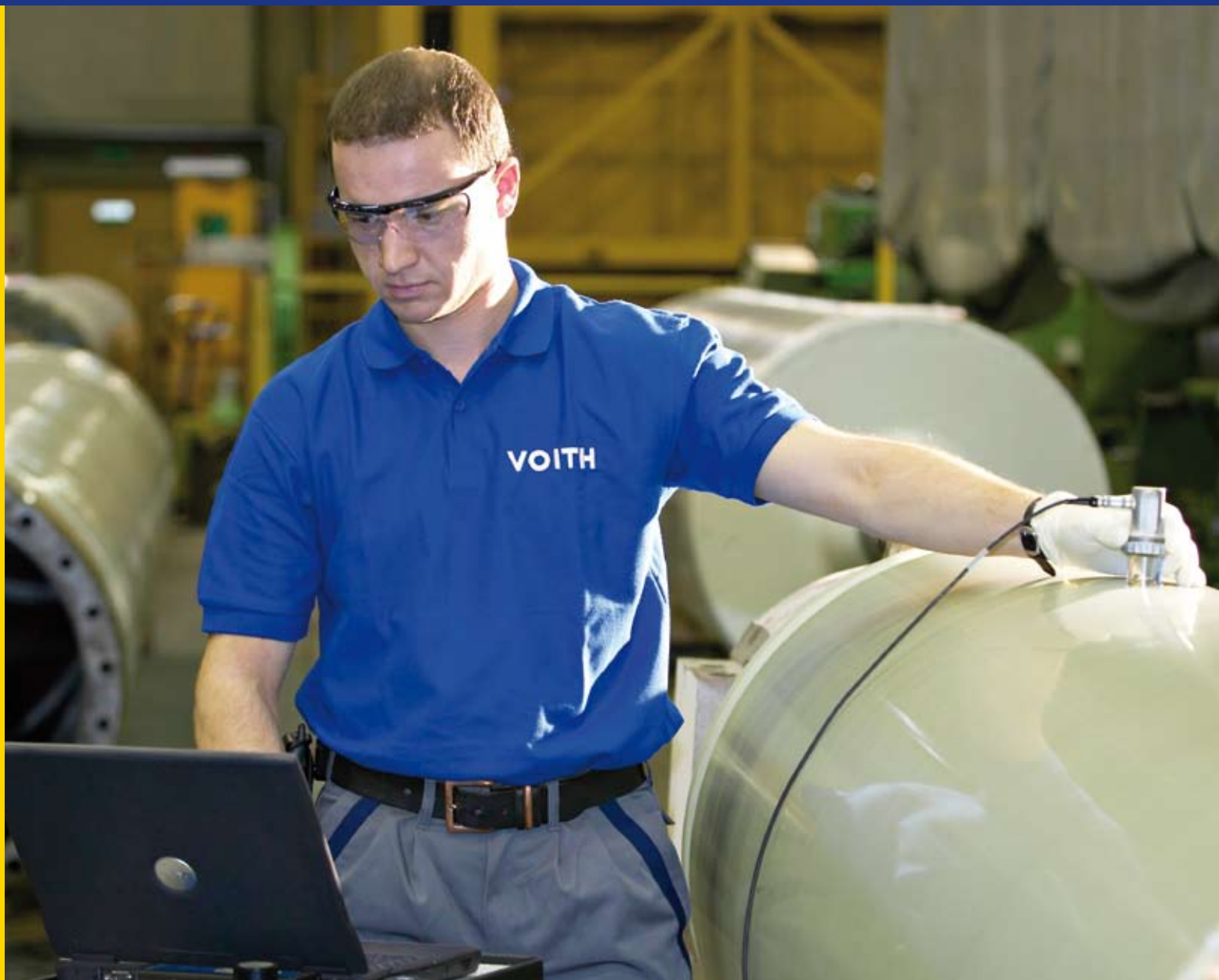
RollCare: Ultrasonic testing of a roll cover.
