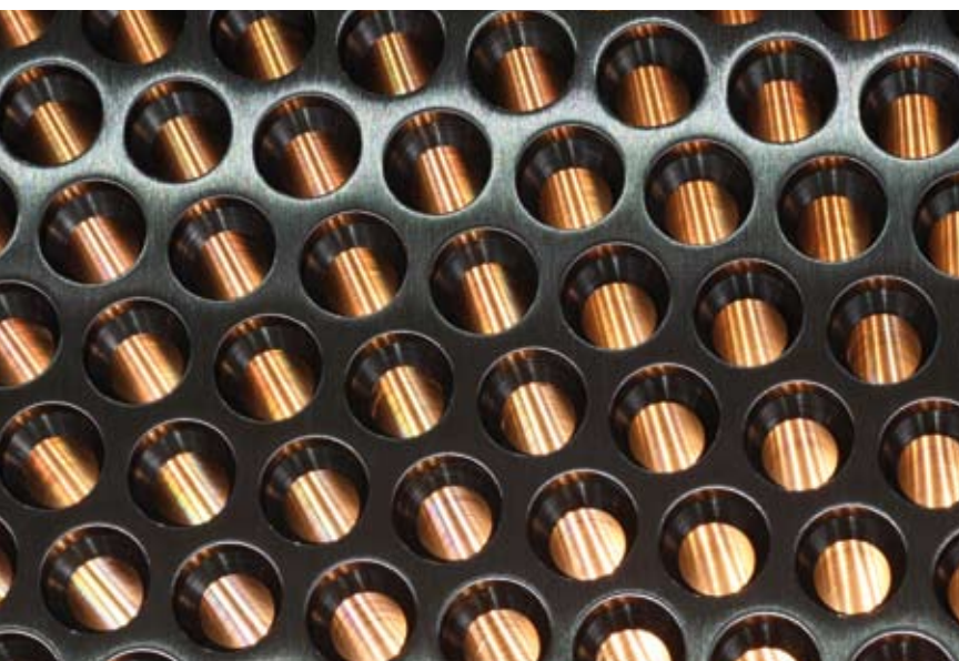
Made to measure: Suction holes are drilled into the duplex steel by spindles.
