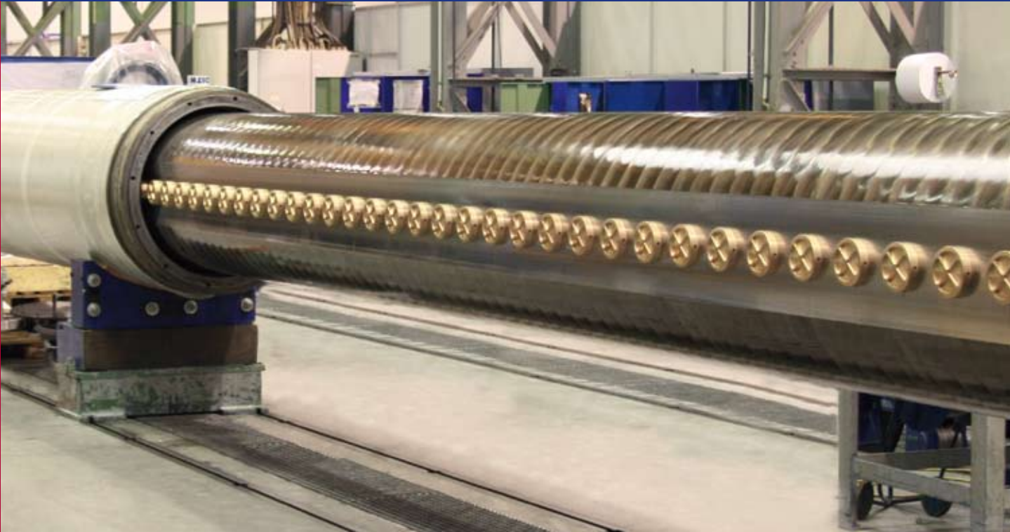
The same Nipcorect roll in the rebuild to counter support elements.
