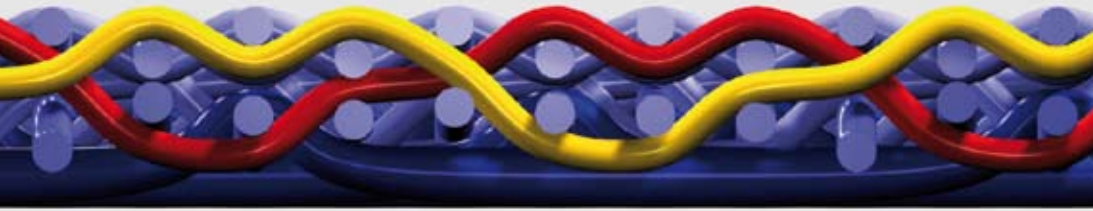
The eight shaft structure on the machine side.
