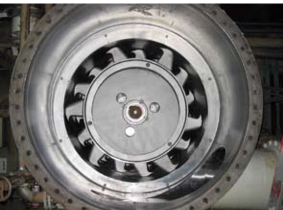
Converted TLA 450 with MultiFoil rotor and C-bar screen basket.
