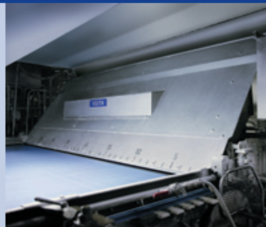
The new headbox under working conditions
