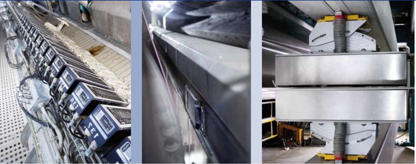
Continuous quality control system from the headbox to the reel: OnQ ModuleJet, OnQ EnviroScan and OnQ Scanner.
