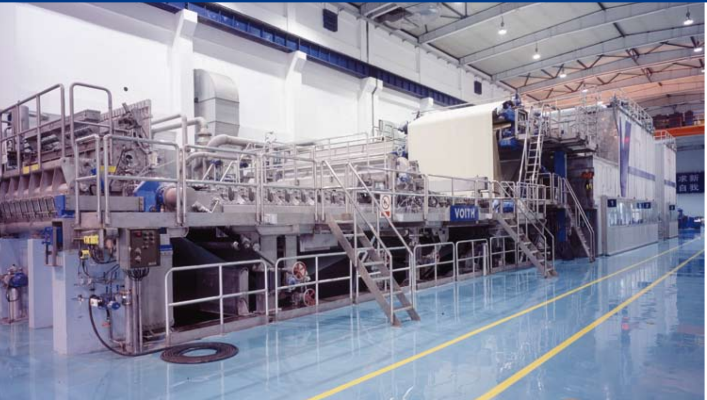
This cigarette paper machine in China produces 12,000 tons of cigarette paper per year.
