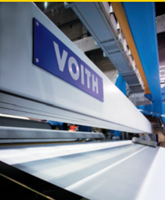
Using data taken by the scanner, OnQ GradeManager monitors the grade change for the paper web's basis weight, moisture and ash content.
