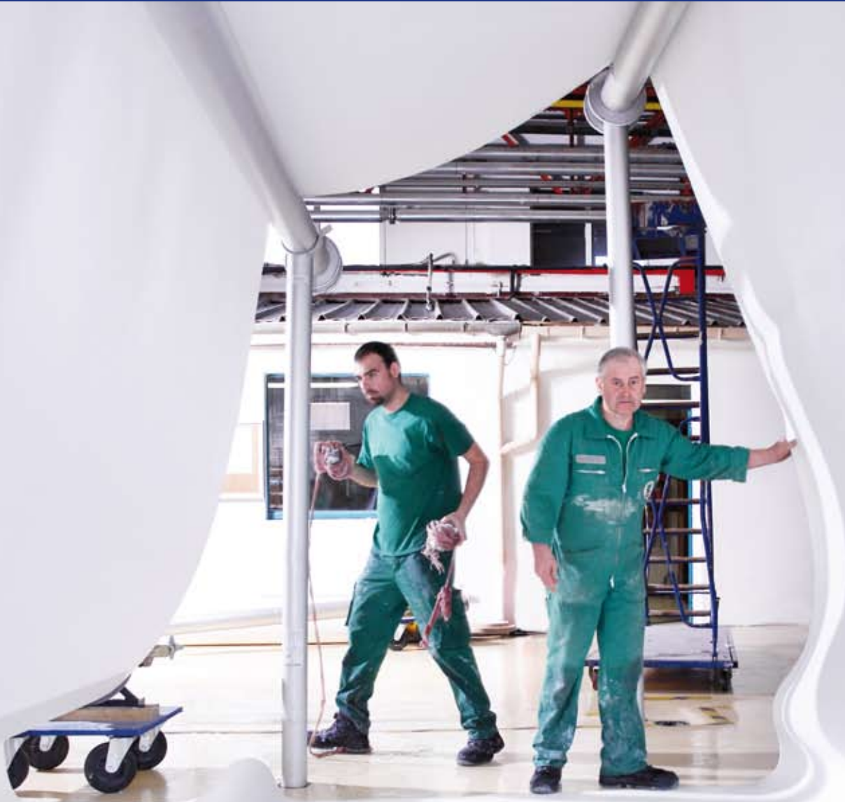
Felt change in Docelles: the bottom felt is prepared for the installation in the press section.
