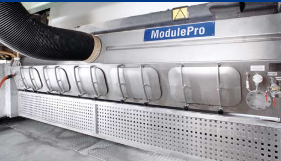
The ModulePro C jet spray dampener moistens the paper web in the coating machine.
