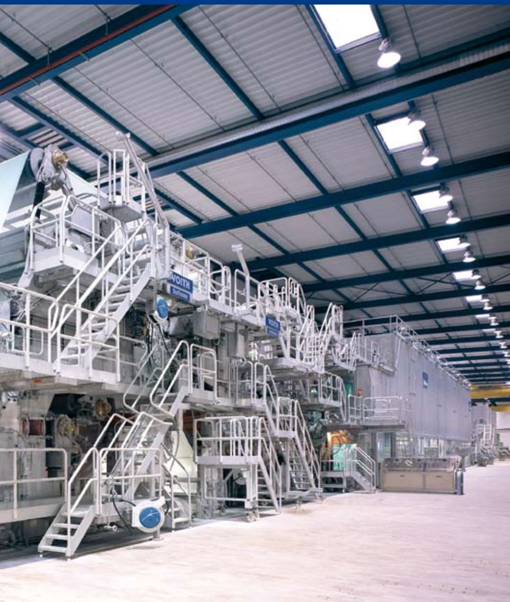
The PM 2 at the Koehler facilities in Kehl is used exclusively for the production of thermo papers in the basis weight range of 40 to 80 g/m 2 and at a production speed of 1,600 m/min.
