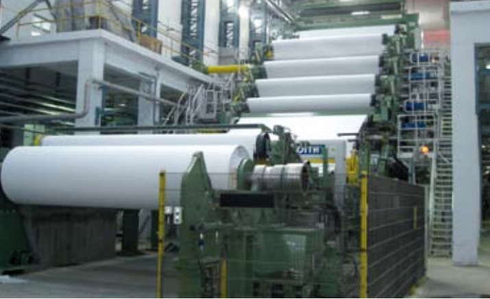
A 10-roll Janus MK2 calender provides for optimum surface treatment.
