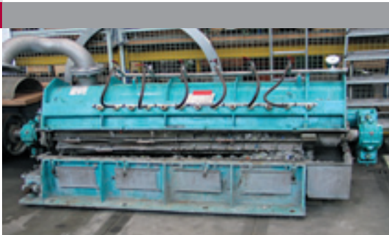
- Rotor and housing heavily damaged
